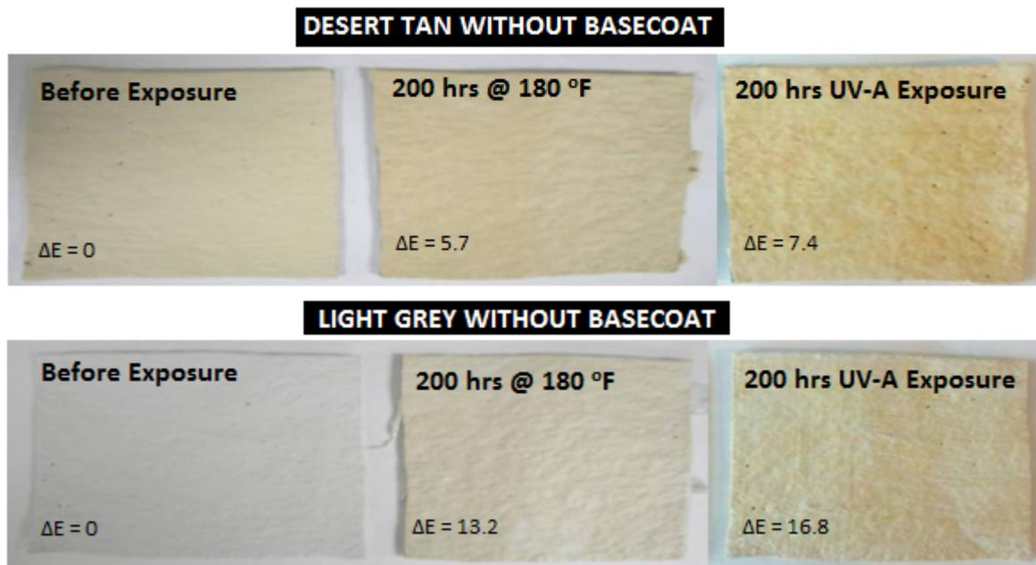
**Figure 2: Images of PERLASTIC with topcoat (no basecoat) before and after heat and UV-A Exposure.**
