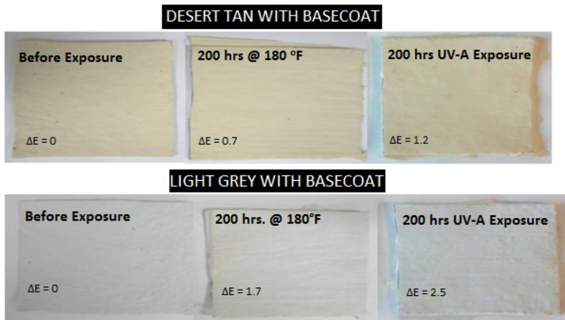
Figure 1: Images of PERLASTIC with basecoat + topcoat before and after heat and UV-A Exposure.
